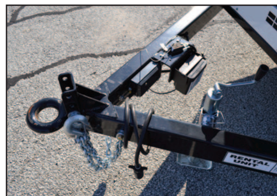
Pintle hitch with electric brakes and 7 pin trailer connector
